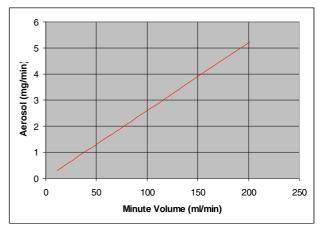
Diagram for rodents at 1.5 bar Mouse Minute volume 20 - 50 ml/min Rat Minute volume 140 - 180 ml/min Guinea Pig Minute volume 130 - 200 ml/min
