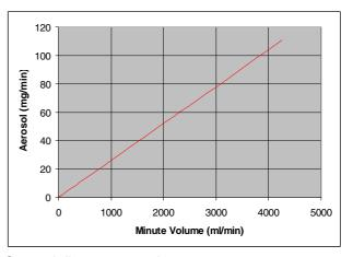
General diagram at 1.5 bar Mouse Minute volume 20 - 50 ml/min Rat Minute volume 140 - 180 ml/min Guinea Pig Minute volume 130 - 200 ml/min Rabbit Minute volume 400 - 600 ml/min Dog Minute volume 3 - 4 l/min
